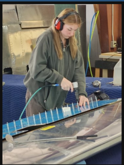
Reagan is riveting the final skin on the wing.
